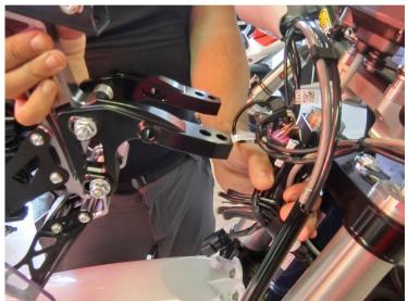
Align is important so check that the cables that need to be in the middle of the tower are there, while the brake line and cables that need to be outside, they stay outside!
