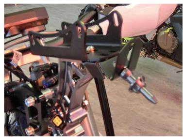
Leave the bolt on the screen holder and the bracket a bit loose until you decide the final position!
