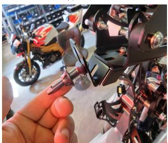
To assist in installing the screen in the pin, you can use a bit of grease inside the grommet. NEVER use WD40 on the screen!
