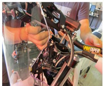
The foam is there to prevent back-scatter and not blind you during night-riding. Due to the screen being able to move, the foam cannot be fully fixed.
