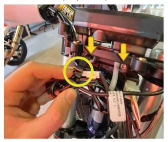
Start removing the connectors from the plastic bracket one by one. Remove the speedometer from its bracket.
